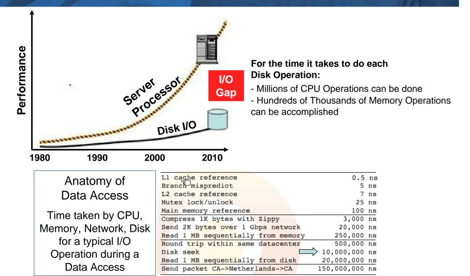
A 7.2K/15k rpm HDD can do 100/140 IOPS
